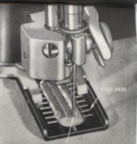
END OF STEP ONE AT 2ND MARK ON RIGHT NEEDLE DOWN IN FABRIC WHILE CLOTH CLAMP IS RAISED AND MOVED
