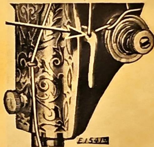
Fig. 2 Threading for Darning on Machines 66 and 99
