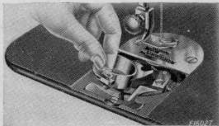
FIG. 22. REMOVING THE BOBBIN CASE
