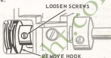
Fig. 39. Removing Hook Assembly
