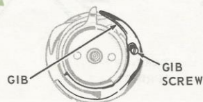
Fig. 38. Removal of Gib Screw and Gib
