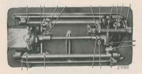
FIG. 27. OILING POINTS IN BASE OF MACHINE
