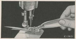
FIG. 42. INSERTING BINDING IN BINDER
