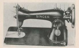
FIG. 23. FRONT VIEW, SHOWING OILING POINTS
