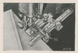
FIG. 51. PROPER POSITION OF MATERIAL IN TUCKER
