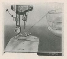
FIG. 13. DRAWING UP THE BOBBIN THREAD
