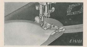
FIG. 45. BINDING AN OUTSIDE CURVE
