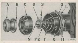
FIG. 20. REASSEMBLING AND REPLACING THE TENSION
