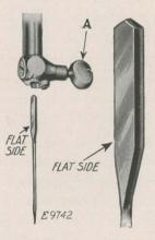
FIG. 11. POSITIONING OF NEEDLE IN NEEDLE CLAMP
