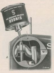
FIG. 24. OILING POINTS AT THE BACK OF THE MACHINE
