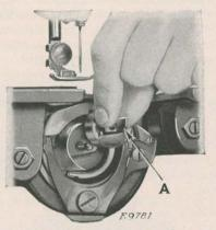
FIG. 4. REMOVING THE BOBBIN CASE
