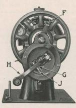
FIG. 3. END VIEW OF MACHINE 15-89 SHOWING THE HAND DRIVING ATTACHMENT
