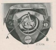
FIG. 10. BOBBIN CASE THREADED AND REPLACED
