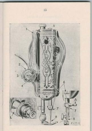
FIG. 12. UPPER THREADING
