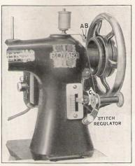
Next, place a spool of thread on the spool spindle nearest the hand wheel, take the end of the thread and pass it downward through open eyelet "A" wrapping one time around the bracket to the left and downward through open eyelet "B", then placing the end of the thread through the hole "C" on the outer edge of the bobbin, holding on to the end until you have run the machine sufficiently to wind
