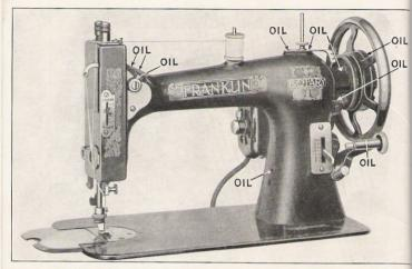
The illustrations above and below show the oiling places on the Franklin Rotary Head.
